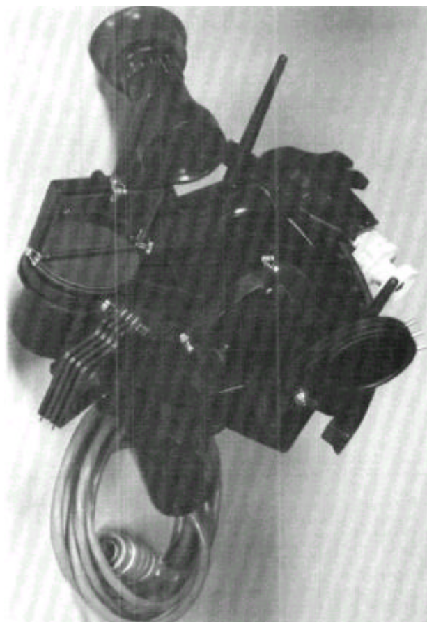
FIGURE AE-3.— Electronic digital sextant
