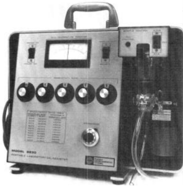
FIGURE AL-7.— Induction-type salinometer (courtesy of Plessey Environmental Systems, San Diego, California)
