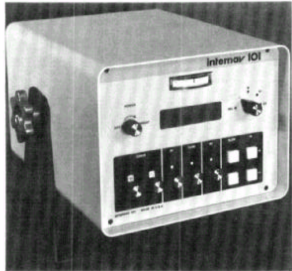
FIGURE AB-3. - LORAN-C shipboard navigation unit (courtesy of The International Navigation Co., Inc., Bedford, Massachusetts)
