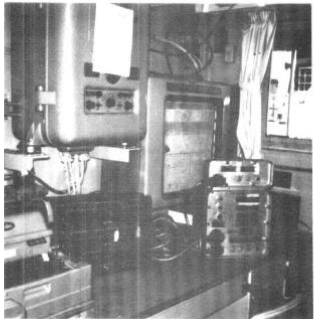
FIGURE AJ-4. — Hydrographic data logger aboard the NOAA ship Davidson
