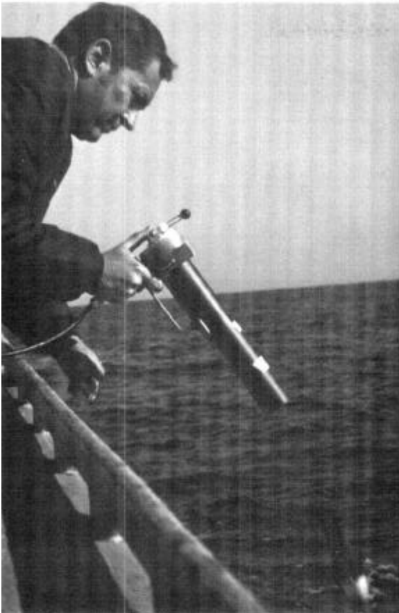
FIGURE AL-12.— Shipek sediment sampler (courtesy of Hydro Products, San Diego, California)
