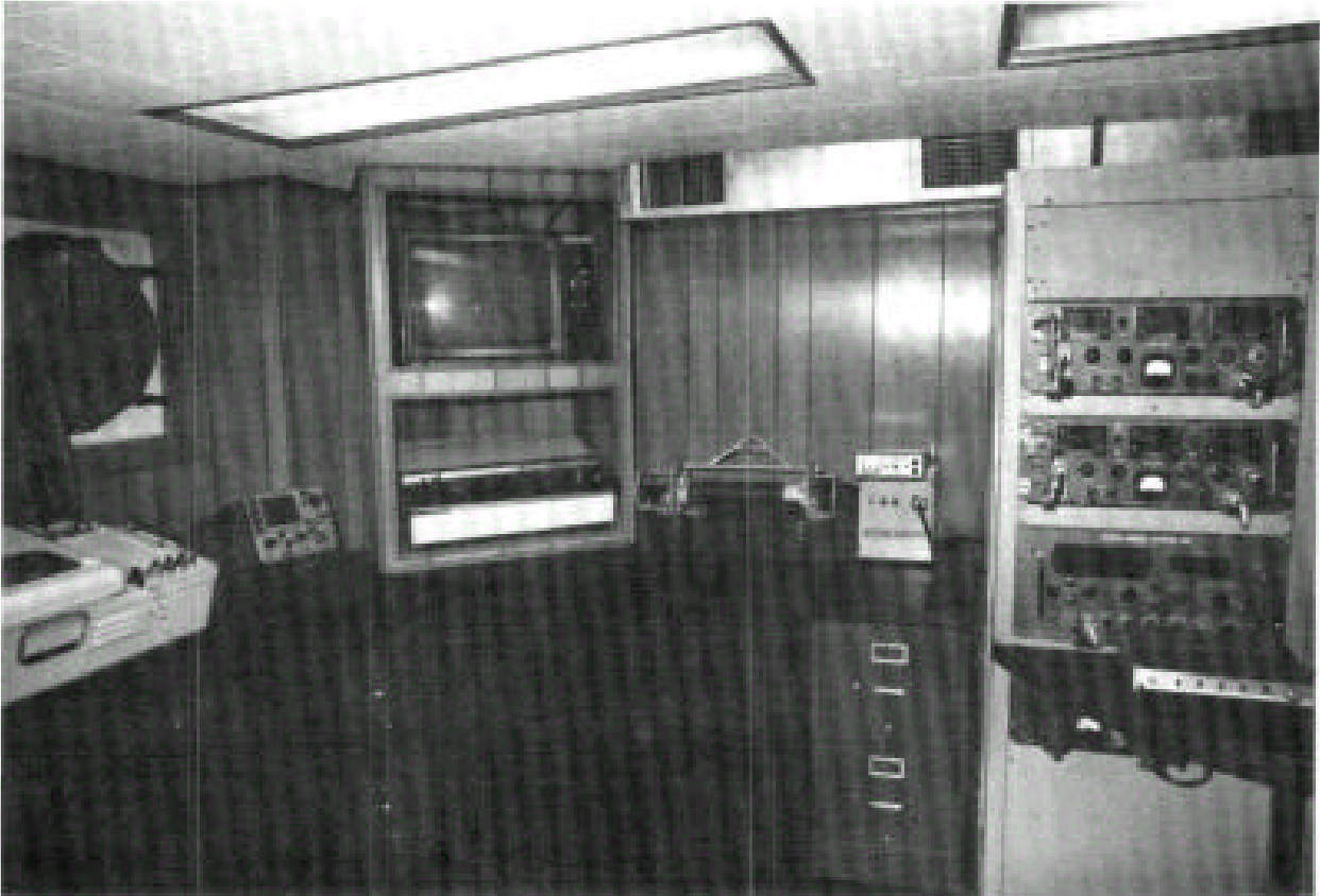
* FIGURE AC-1.-Decca Sea-Fix positioning system shipboard installation ( courtesy of Decca Survey Systems, Inc; * Houston, Texas)
