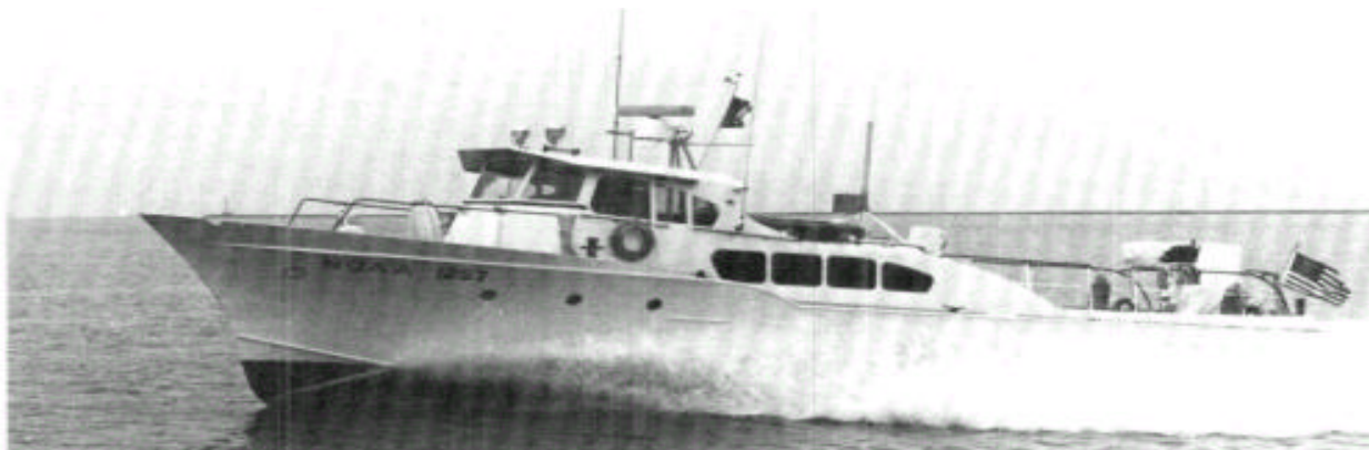
FIGURE AA- 2.— NOAA launch 1257, a high-speed (20-kt) hydrographic survey vessel.
