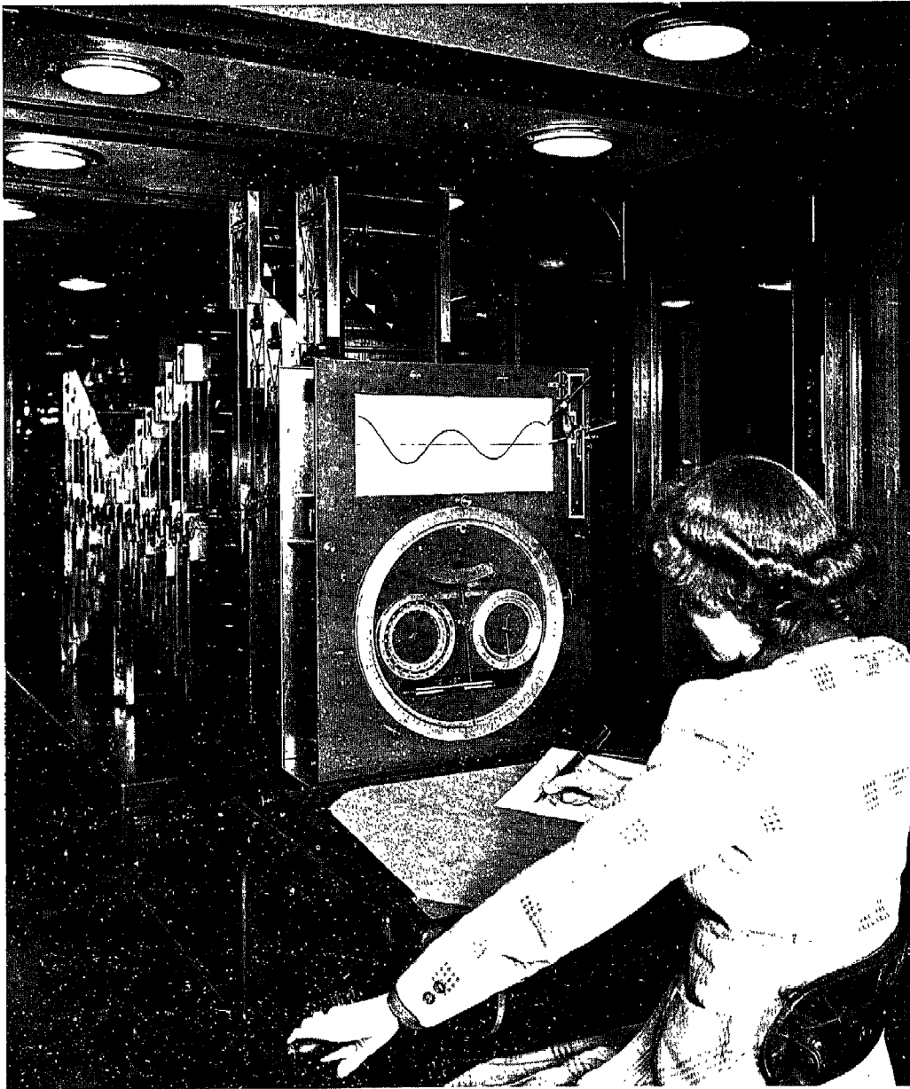
FIGURE 22.—Tide Predicting Machine, designed in the Coast Survey, for predicting the times and heights of the tide for any port in the world and for any year. Astronomical equations involving as many as thirty-seven factors are solved mechanically to produce the tide in nature. Not shown in the view is a recent attachment which automatically types the predictions in the format of the Tide Tables .
