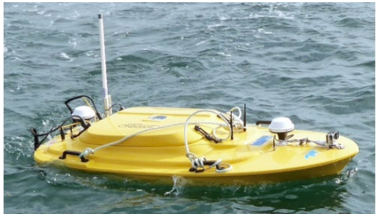
Figure 14. The uncrewed Z-boat, with multibeam sonar, is one option to choose from on surveying shallow waters for NOAA's coastal mapping program and to fill voids from topobathy lidar where waters are too turbid for full bottom coverage.
