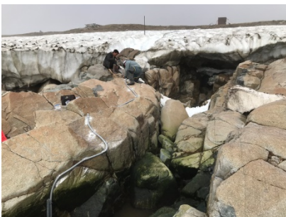
Figure 8. Picture of a vented pressure tide gauge installed for tidal datum determination on St. Lawrence Island, Alaska. Field crew is securing air hose that runs from below MLLW to the electronics enclosure on top of the hill in the background.
