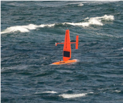
Figure 16. Although the Sairdrones operating in the Arctic are equipped with single-beam sonar, options are available also for multi-beam sonar.
