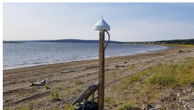
Figure 12. GNSS-Reflectometry water level system installed in Koyuk, AK by JOA Surveys, LLC in support of the NOAA Office of Coast Survey Project OPR-R385-KR-20. TerraSond Ltd. was the prime contractor. Photo courtesy of JOA Surveys.
