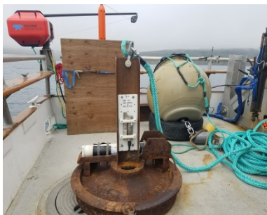
Figure 9. Non-vented pressure, conductivity and temperature sensors secured to an oceanographic anchor prior to deployment south of the Alaska Peninsula.
