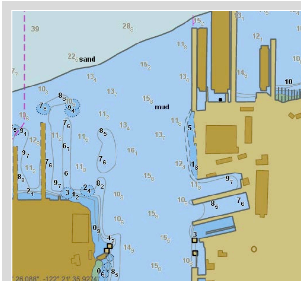
Figure 11 – Safety contour set to 10M. This will cause an unnecessary ECDIS alarm as a ship enters a deep port. Because no 10 m depth contour is available, ECDIS will portray the next shoaler available depth area (30 ft, 18.2m) as “unsafe water.”
