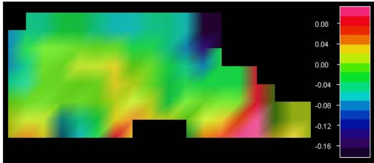
Figure 3c – Difference surface between ERZT and VDatum for NOAA H12216 [height in meters]
