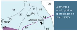
Figure 4. Examples of cartographic representations of unverified hazards to navigation.
