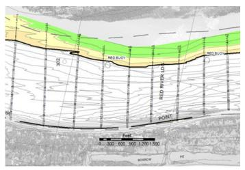
Figure 2. USACE condition survey showing lines of depth measurements approximately 200 meters (656 feet) apart.
