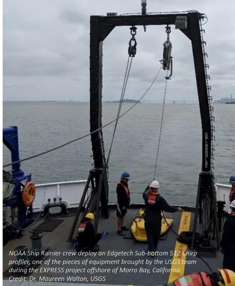
NOAA Ship Rainier crew deploy an Edgetech Sub-bottom 512 Chirp profiler, one of the pieces of equipment brought by the USGS team during the EXPRESS project offshore of Morro Bay, California. Credit: Dr. Maureen Walton, USGS
