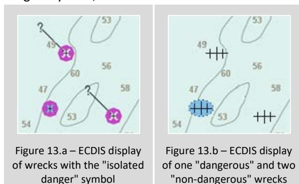
Figure 13.a – ECDIS display of wrecks with the "isolated danger" symbol
