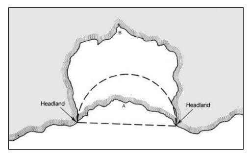
Figure 48. The semicircle test. Applying the semicircle test, indentation "B" qualifies as a bay, but indentation "A" does not. (After I Shalowitz, Figure 4)
