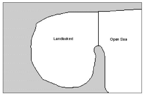
Figure 59. Shortest distance test. The shortest distance test is applied to determine where internal waters are enclosed by one distinct headland and a straight coast opposite.
