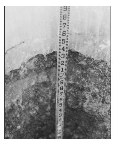
Figure 36. Ice/gravel mix in subsurface of Dinkum Sands, Alaska. The U.S. contended that ice should be discounted in calculating the feature's elevation. (*Photo by Dr. Erk Reimnitz*)
