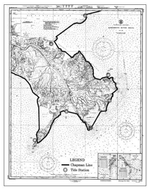
Figure 84. Portion of the Chapman Line on the Mississippi River delta. The line was constructed using pre-Convention principles. (From I Shalowitz, Figure 23)
