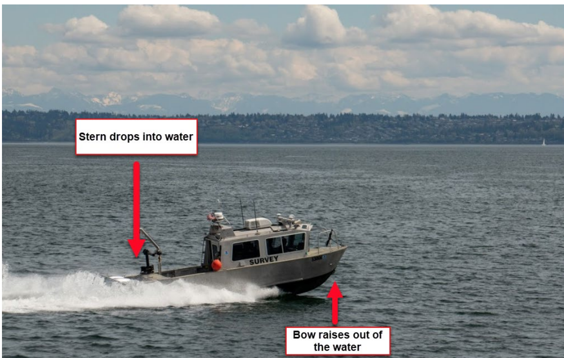
FIGURE 1-1 SQUAT AND SETTLEMENT AFFECT THE SONAR’S VERTICAL LOCATION. AS THE VESSEL INCREASES SPEED, THE SONAR’S VERTICAL POSITION LOWERS IN THE WATER.
