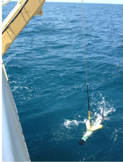
FIGURE 1-8 EXAMPLE OF LAUNCHING A TOWED SIDE SCAN SONAR ON NOAA SHIP THOMAS JEFFERSON
