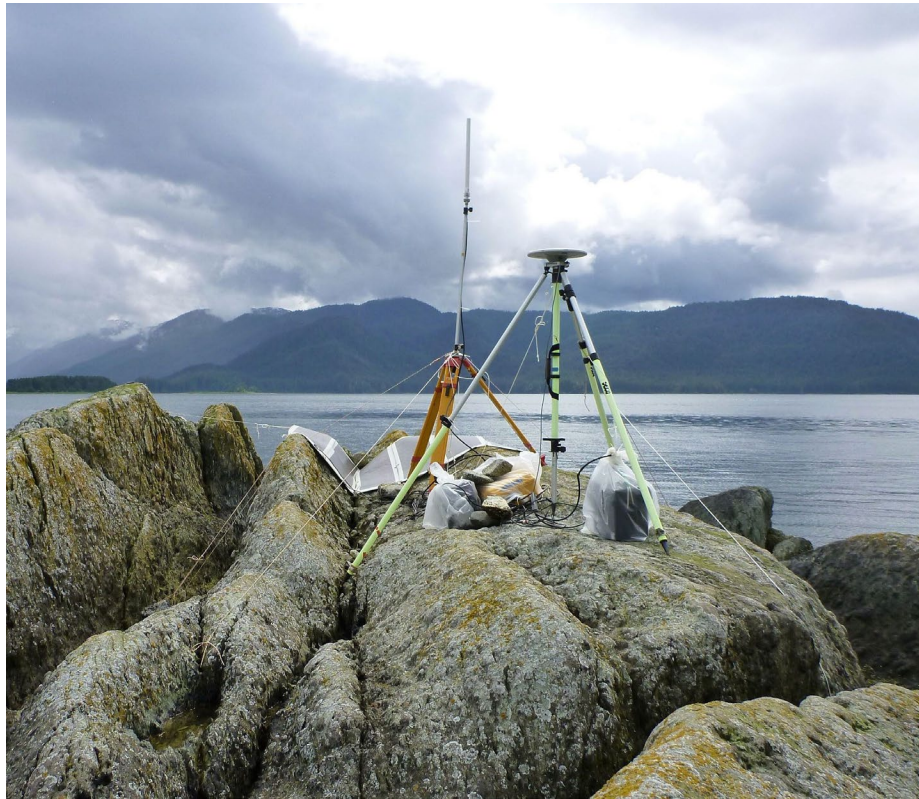
FIGURE 3-4 GNSS REFERENCE STATION SET UP BY NOAA SHIP RAINIER
